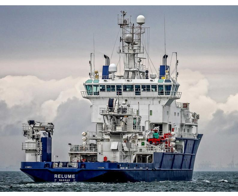
The MPSV levoli Relume is a DP2 vessel with an ample working deck, a 25-tonne crane and advanced survey equipment. This multitask specification ensures that the Relume is able to fully service a diverse range of maritime needs, including offshore operations.
