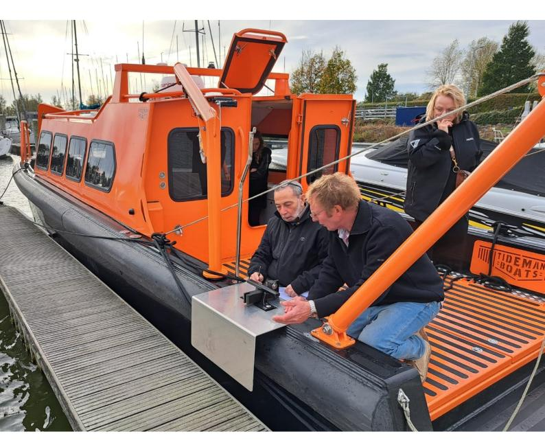
The ASV NG COASTAL is a solid 10,7m long brand new low-draft coastal survey boat specifically designed for nearshore marine surveying and is outfitted with modern positioning, bathymetric, geophysical, geomorphological and geotechnical equipment. She can also be successfully utilized for observation class ROV inspections and oceanographic investigations.
